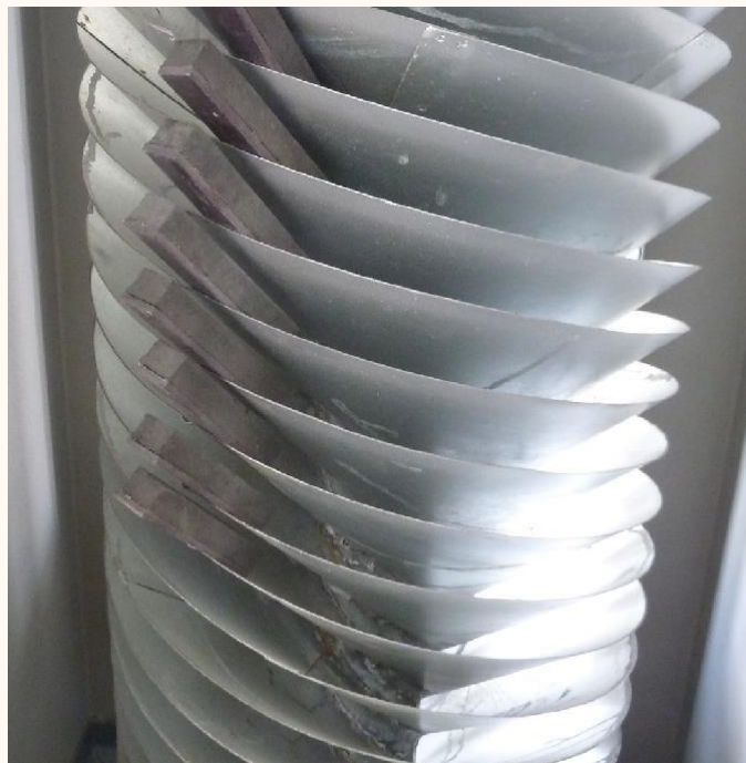
Figure 3: Seed dams for slowing down the crop flow on the same level in all eight flights.
