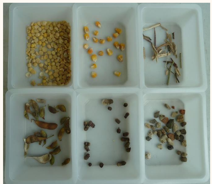
Figure 5: Impurities with which the tests were carried out. The samples come from various Taifun soy deliveries.
