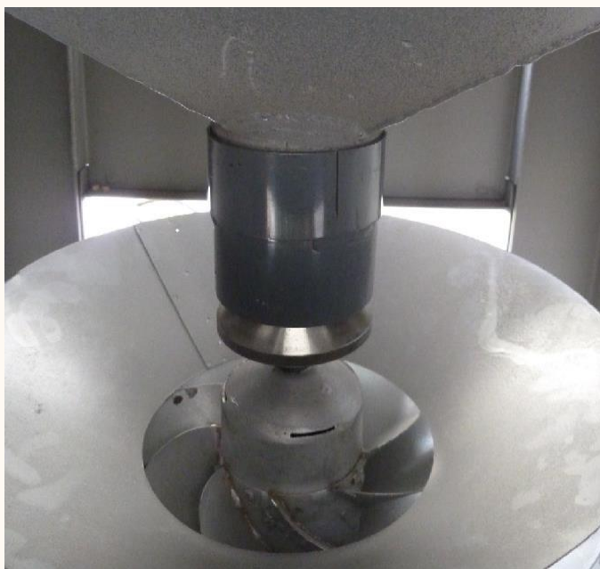
Figure 2: Screw cone for dosing and even distribution to the eight spirals
