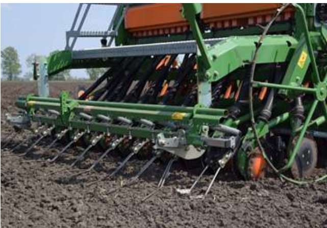
Amazon grain drill, with gravity seed metering/delivering mechanism, provides row width of 150 mm. Photograph: Donau Soja Ukraine
