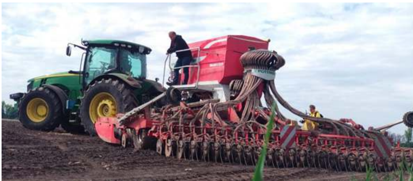
Grain sowing complex Pöttinger, with pneumatic seed metering/delivering mechanism, provides row width of 125/167 mm, or 250 mm. Photograph: Mykola Bykov (Donau Soja Ukraine)
