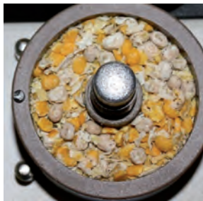
Fig. 2.6 b: Measurement of the moisture content of a lupin sample with 16.5%
