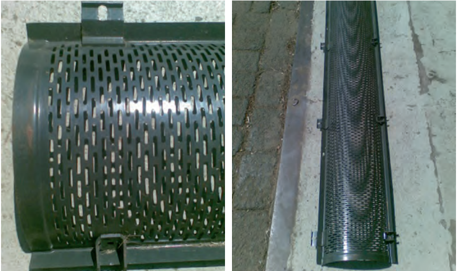
Fig. 2.4: Inserting of a special sieve into the transverse auger of the combine harvester (perforated Claas grain pan).
